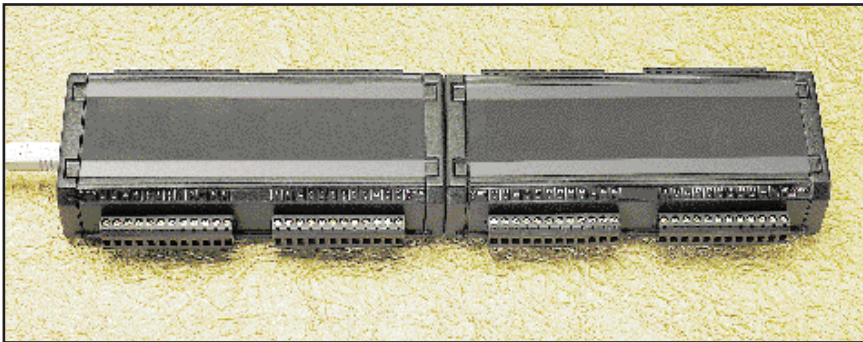
An OMB-DAQ and a PDQ module simply plug together for additional channel capacity
